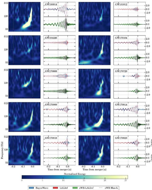
**Figure 5:** Time frequency maps and reconstructed signal waveforms for the ten binary black hole events reported in our catalog. In the right hand panel for each detection, the different colors represent different methods for reconstructing the waveforms; these are found to be consistent with each other when we take into account the uncertainties in the process. (Adapted from Figure 10 of our [paper](#).)
