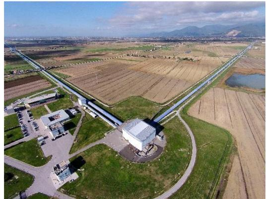
*Aerial view of the Virgo gravitational-wave detector, situated at Cascina, near Pisa (Italy). Virgo is a giant Michelson laser interferometer with arms that are 3km long. (Image credit: Nicola Baldocchi / The Virgo collaboration)*
